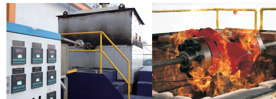
Fire safe Test equipment
