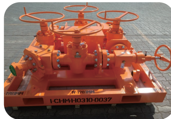
Well testing manifold in Iraq
