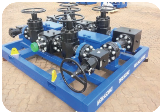
Well testing manifold in Saudi
